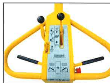
Multi-functional handle controls forward and reverse travel, water flow to the drum, vibration and the emergency stop feature.
