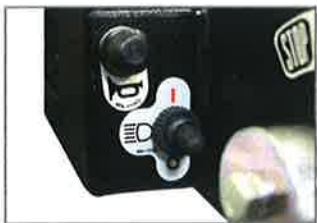
Horn and headlight switch for job-site safety
