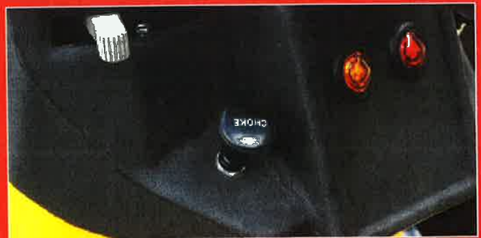
Dashboard with slide throttle control, 2 indicator lights, integrated choke and waterproof ignition.
